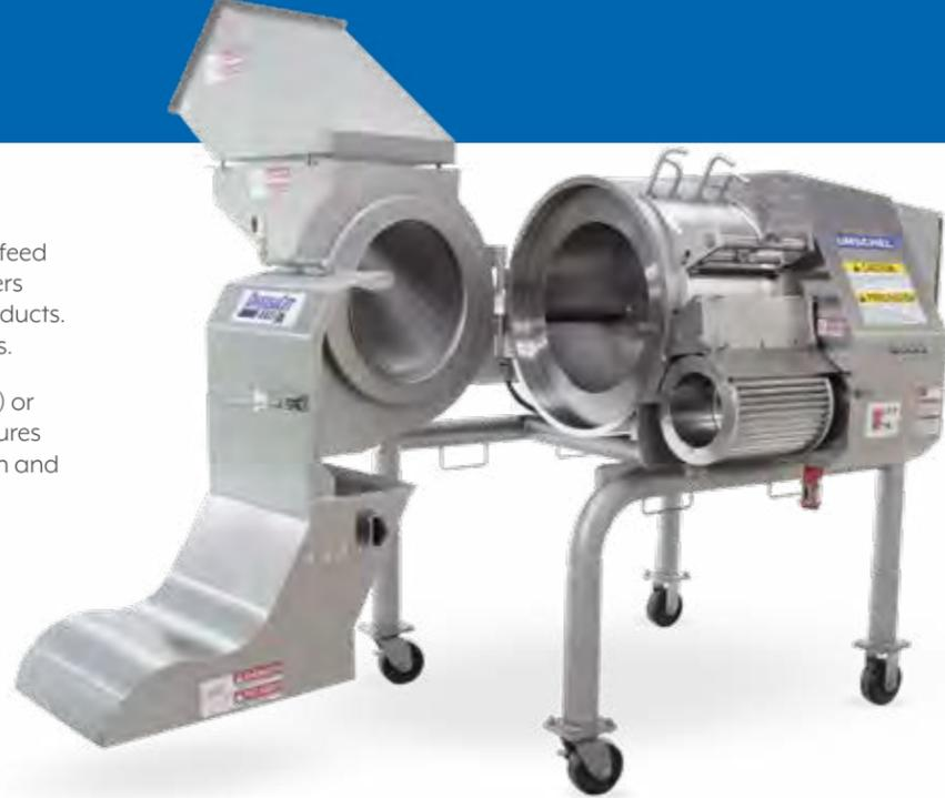
**Cutting zones are completely separate from mechanical zones.** Rounded tube frame contributes to sanitary design and eases cleaning.
