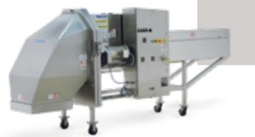
The TranSlicer® Cutter is introduced (later renamed the TranSlicer 2500). It revolutionizes the fast-growing salad industry with its ability to accept up to a 6" head of lettuce and uniformly cut it for bagged lettuce on grocery shelves.
