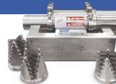
The Flo-Cut Model 360 cutting head is designed for use in large volume watergun systems. This unit can be integrated into watergun systems and offers fast, easy cutting head replacement for changing knives or sizes of cuts. Infeed diameter measures 3.375" (86 mm) and a discharge diameter measures 5.820" (148 mm). The Model 360 is designed for easy cleanup and maintenance.
