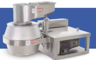
Lattice slicing is a unique application. Proper feeding of the machine is necessary to ensure continuous production. Tempered high quality oval or flat shaped potatoes measuring between 2 – 4 inches (51 – 102 mm) are best-suited. Model CC Slicers can be converted to Model CCL Lattice Slicers.
