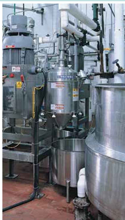
Uniform milling of poultry skin is finished on two Model 1700's for the production of a soup base.
