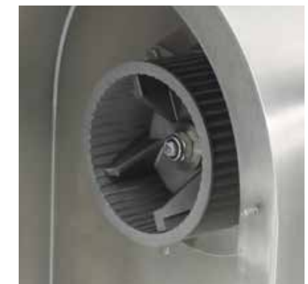
Cutting unit with cutting enclosure removed (for illustration)
