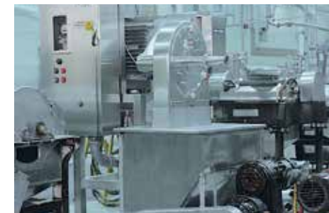
Model 9300 is used to mill fruits and vegetables into a fine puree for production of baby food.
