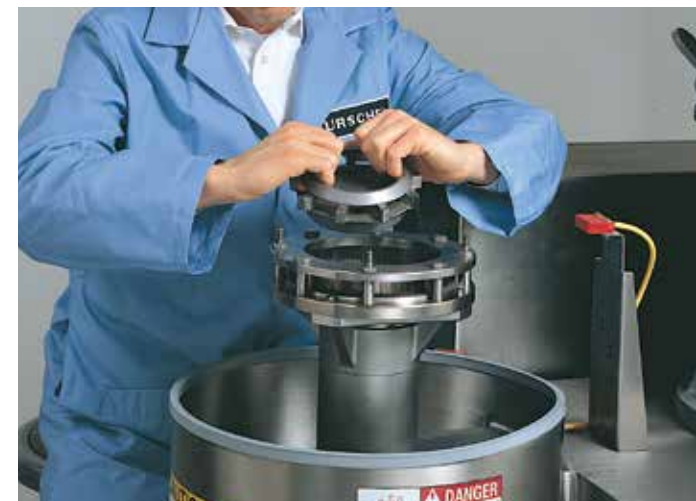
Impellers and Microcut Heads are easily changed to facilitate other applications, cleaning, or maintenance.
