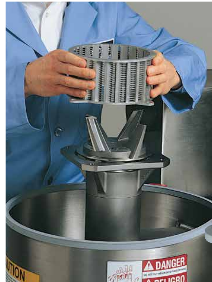
Cutting heads and impeller are easily changed to facilitate other applications, cleaning, or maintenance.
