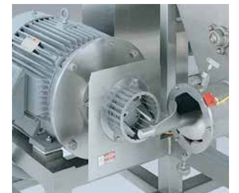
Cutting unit with cover removed (for illustration)
