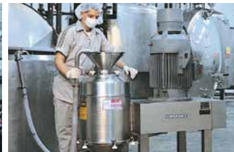
Aloe vera is milled on the Model 1700 for use in a variety of dermatological products.
