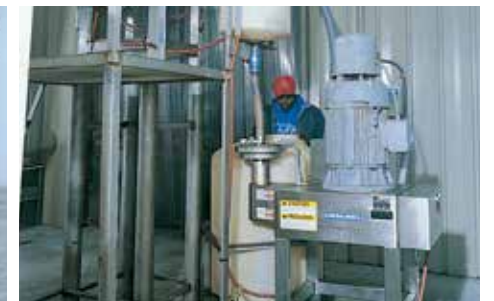
Peppers are uniformly produced in a two stage milling operation using two Model 1500 units.
