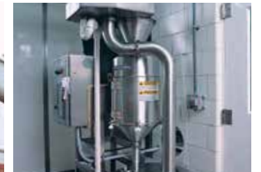
Poultry skin is precut on a Model 1700 equipped with a cutting head.
